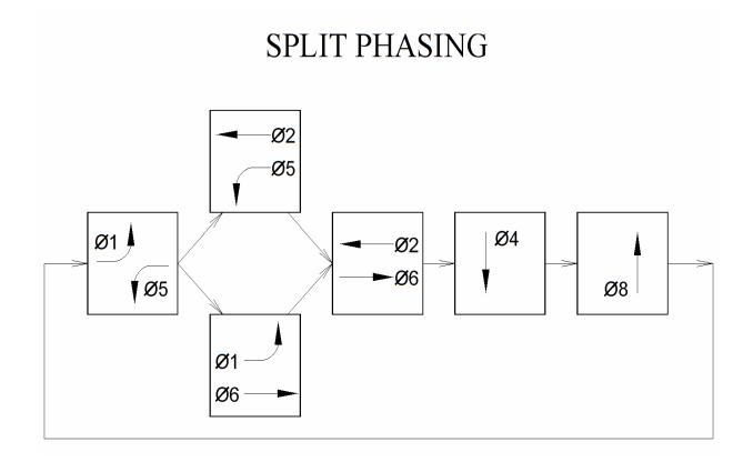
Split phasing is frequently used at intersections with offset (staggered) side street approaches or where the existence of shared thru/left lanes makes it impractical to use an exclusive left turn phase.
