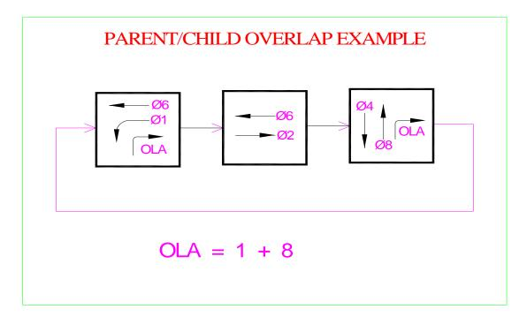
This right turn arrow would be called either a "1+8" overlap or an overlap with phase 1 and phase 8 parents.
