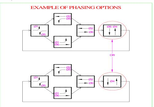
Split phase operation is a type of phase rotation which does not have exclusive left turn phases on the side street, and which services each of the side street phases separately, rather than simultaneously. As with quad phasing, the left turns on the main street operate concurrently with the opposing left turn and with the adjacent thru phase.
