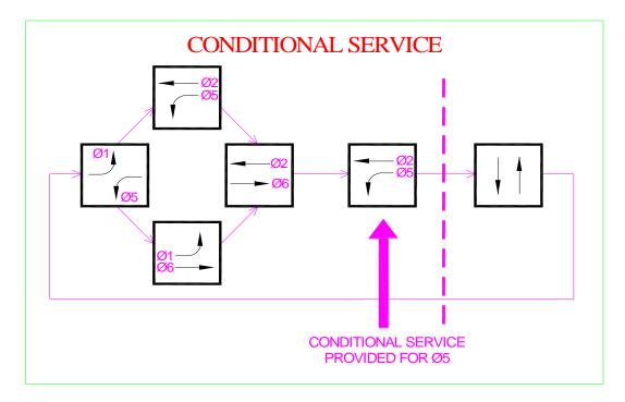
The left turn that has been placed into conditional service can be served twice during the phase rotation. Activating conditional service for a left turn phase does not guarantee that the phase will be served twice every cycle. If the opposing thru traffic is heavy enough, then the left turn phase will only be serviced once during that cycle.
